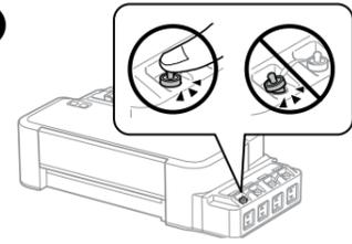
Make sure to close the cap onto the ink tank securely.
