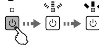
**8** Press for **3 seconds** until the light starts flashing. Charging ink is started.
