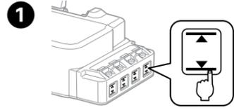
Check the ink levels. If the ink level is below the lower line, refill the ink.
