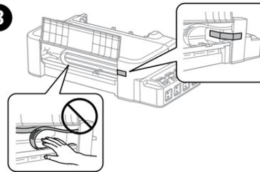
Open the front cover and secure the print head with a tape.
