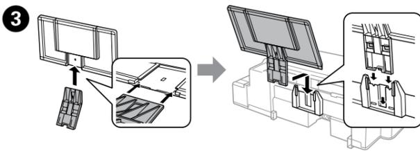
Connect the parts and attach the paper support.
