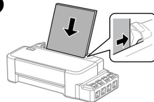
Load the paper with the printable side up.
